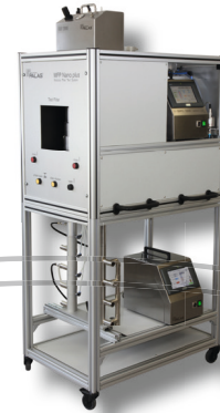
MFP Nano plus filter media, pressure mode, for droplets and salts, MPPS range with U-SMPS 2050
