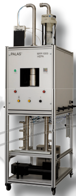
MFP 1000 HEPA filter media, pressure mode, for droplets and salts, MPPS range
