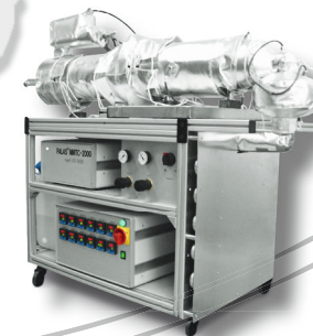
MMTC 2000 EHF for cleanable filter media according to VDI 3926 with humidity and temperature control
