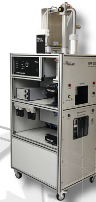
MFP 3000 filter media, suction mode for powders, droplets and salts C_{m \max} \approx 1 \text{ g/m}^3 with welas® digital 3000 gravimetric efficiency
